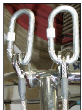
▲ Rigging Of Frame Type 'D'
