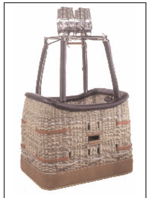
▲ Chaize Basket Fitted With Double Shadow Burner
