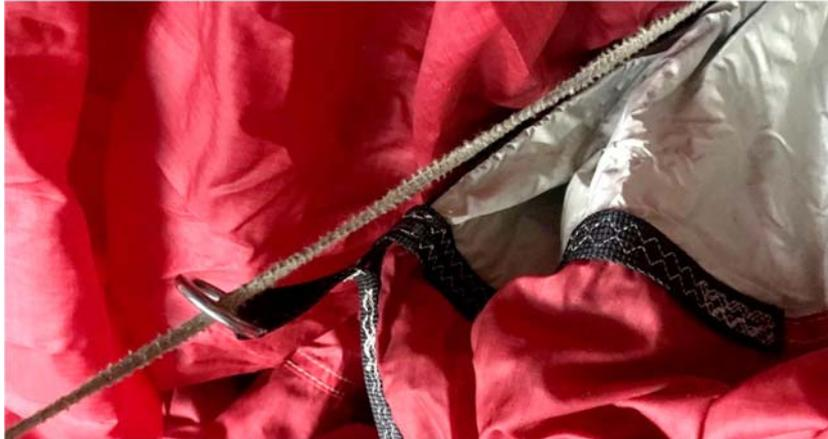
If the length of control cord that passes through the metal ring is significantly worn compared to parts of the control cord that do not pass through the ring, the control cord must be replaced.
