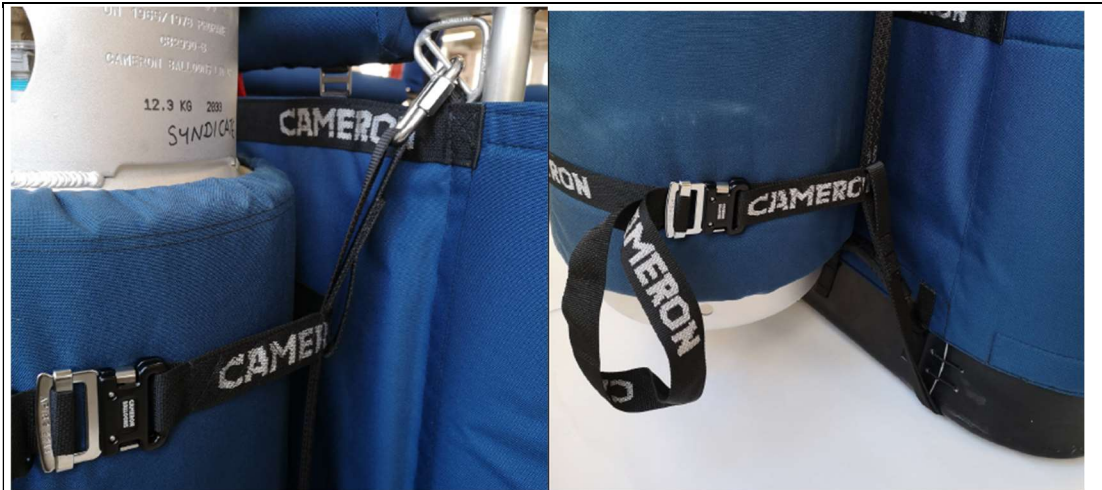
Figure 8 - shows the correct rigging of upper and lower cylinder straps.
